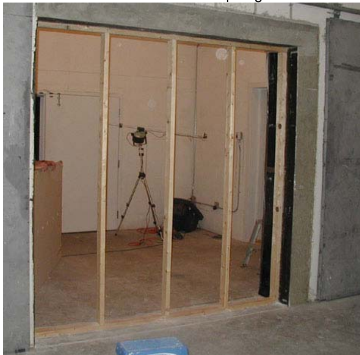
Figure 1: Wood stud frame mounted in test opening
